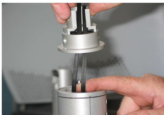
Imagen 8. Belt between rollers and tensioner wall
